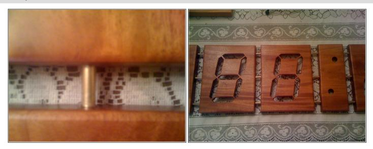
• Connect the digits together using brass tubes and super glue.
